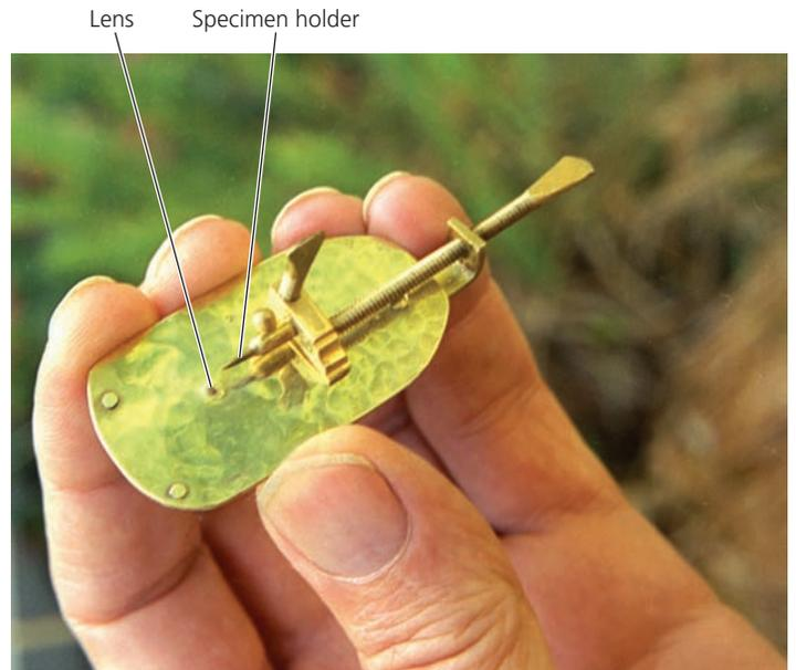
▲ **Figure 1.2** Reproduction of Leeuwenhoek's microscope. This simple device is little more than a magnifying glass with screws for manipulating the specimen, yet with it, Leeuwenhoek changed the way we see our world. The lens, which is convex on both sides, is about the size of a pinhead. The objective to be viewed was mounted either directly on the specimen holder or inside a small glass tube, which was then mounted on the specimen holder.
