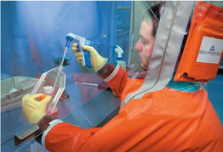
▲ **Figure 25.35** Working in a Biosafety Level 4 lab. The “space suit,” which is designed to completely prevent contact with pathogens, constitutes more than a physical barrier; should the material of the suit be breached, positive air pressure within the suit ensures that pathogens present will be blown back from the opening.
