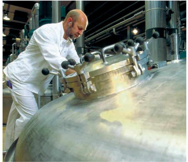
▲ **Figure 26.5** Fermentation vats. Such large containers are used for growing microorganisms in the vast quantities needed for the large-scale production of many industrial, agricultural, and medical products. Why are industrial fermentation vats made of stainless steel instead of wood?
