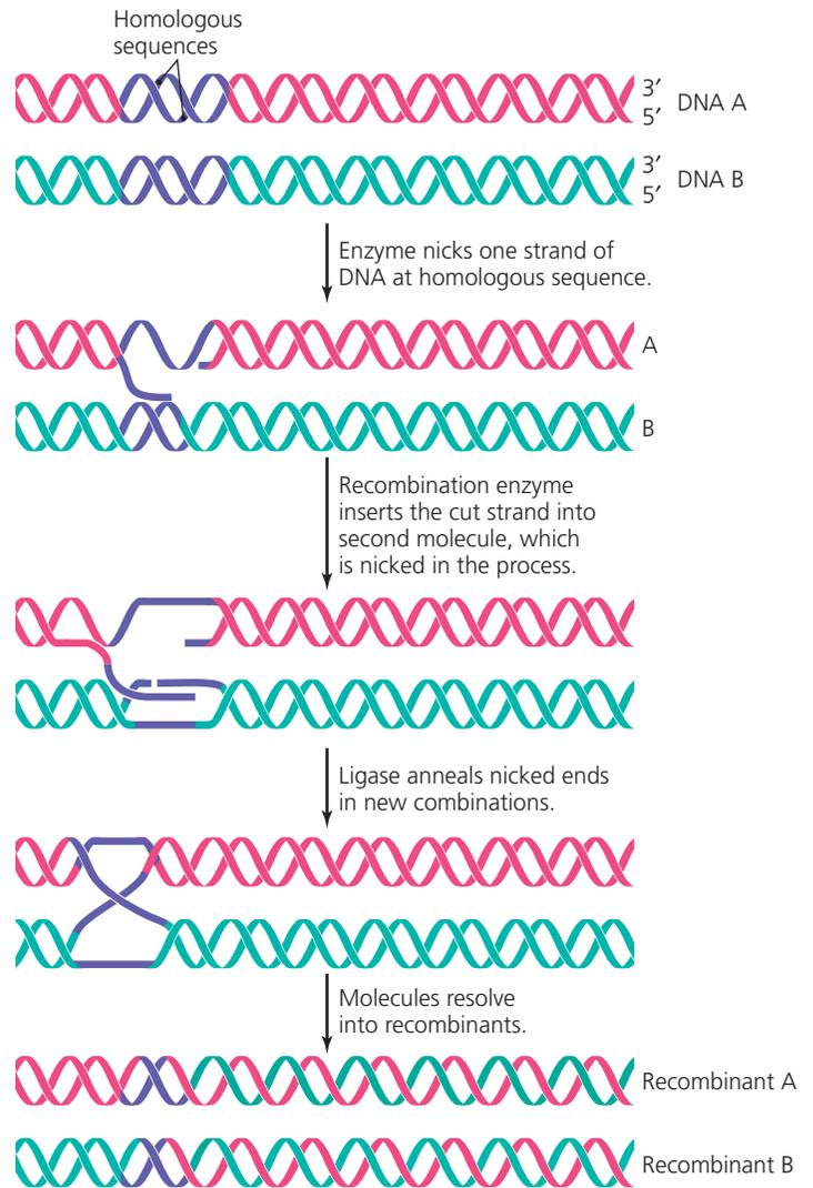
▲ **Figure 7.32 Genetic recombination.** Simplified depiction of one type of recombination between two DNA molecules. After an enzyme nicks one strand (here, strand A), a recombination enzyme rearranges the strands, and ligase seals the gaps to form recombinant molecules. What is the normal function of ligase (during DNA replication)?
